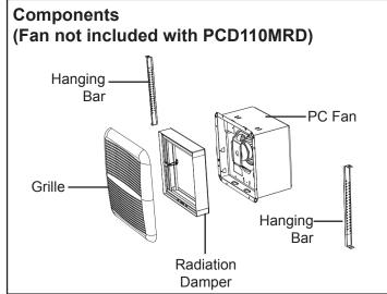
Note: Fan shown is not the PCD110M or PCD110MH
