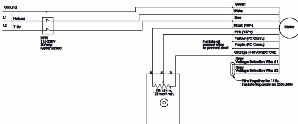
Wiring Diagram For eRED 115V Single Phase and Potentiometer
