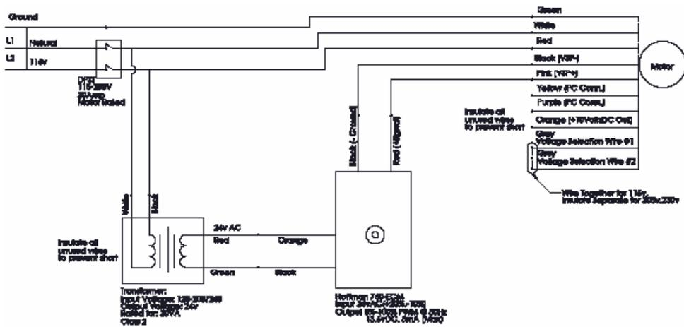
Wiring Diagram For eRED 115V Single Phase with Speed Control
