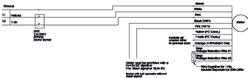
Wiring Diagram For eRED 115V Single Phase less controller
