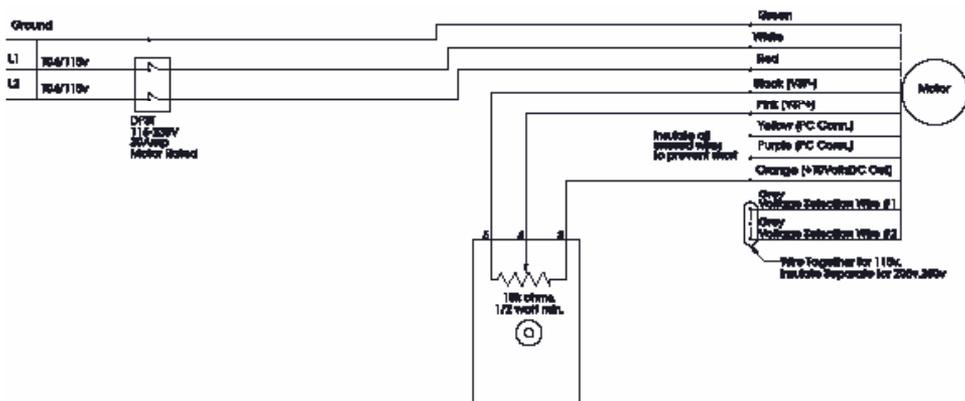
Wiring Diagram For eRED 208/230V Single Phase and Potentiometer
