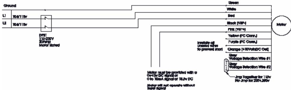
Wiring Diagram For eRED 208/230V Single Phase less controller
