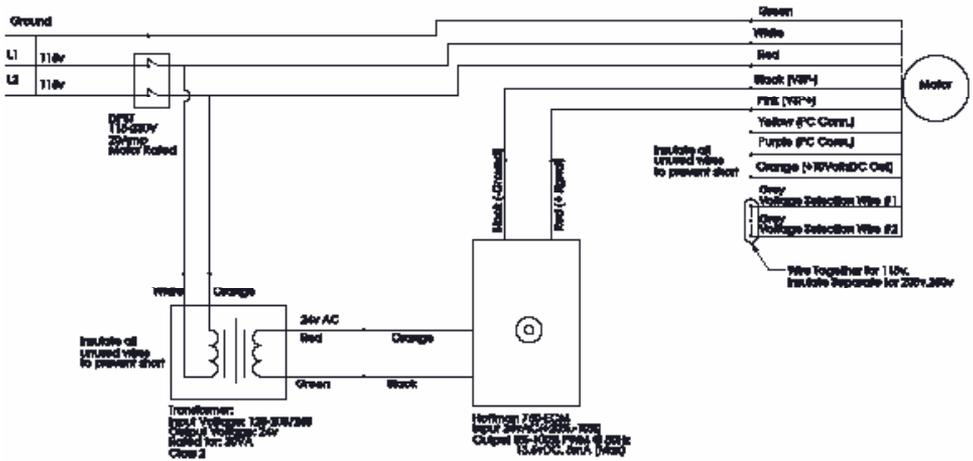
Wiring Diagram For eRED 230V Single Phase with Speed Control
