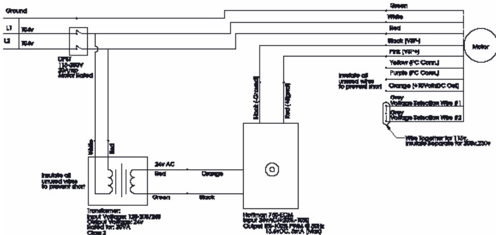
Wiring Diagram For eRED 208V Single Phase with Speed Control
