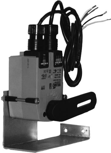
The Model MTR-ACL is an optional 100-240 VAC 50/60 Hz power open spring return motor kit. The adjustable rear blades will return to the closed position in the event of loss of power. The motor kit comes pre-assembled for easy installation.
